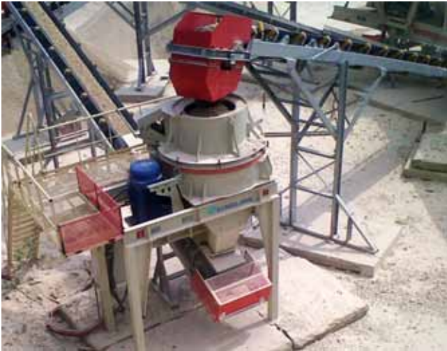
The Kinglink KL-Series VSI's roof lifter allows easy access for servicing the machine, ensuring minimal downtime.
