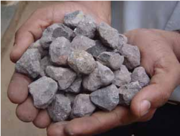
The Kinglink KL-Series Vertical Shaft Impact Crusher can produce high volumes of cubically shaped product.
